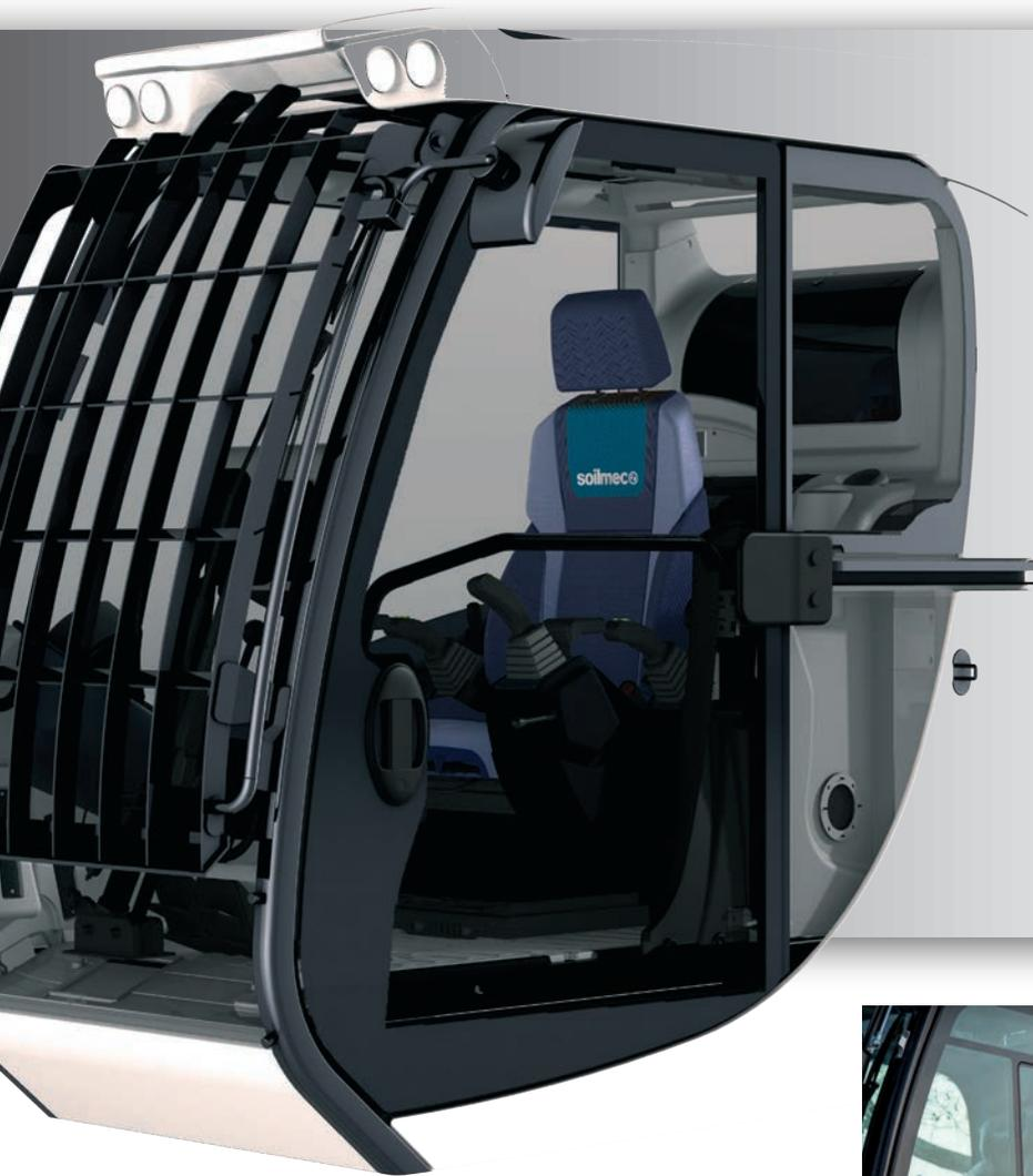
The ergonomic H-cab model embraces the operator. A unique solution in this category (1050 mm /41.6 in wide) in which several accessories facilitate the work of the operator.
