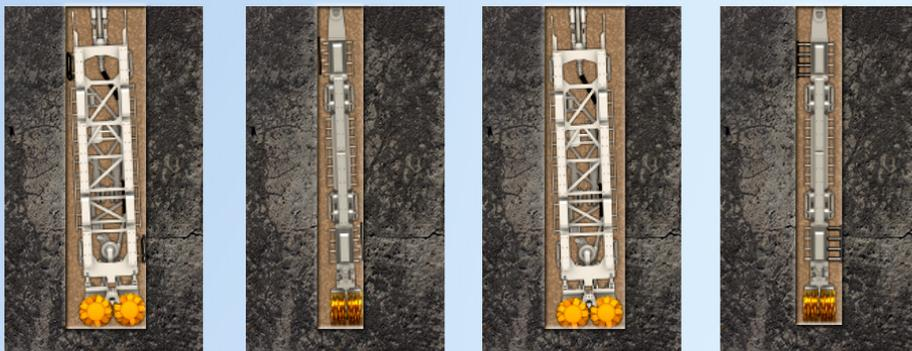
Soilmec Hydromill Verticality Control has been developed in order to reach the best requirements in terms of diaphragm precision, allowing verticality error less than 0,2 % tested up to 250 m depth. Verticality control has been ensured by the means of double or triple axis sensors; for very high depth panels Soilmec defines a special triple axis sensor that guarantees an incredible accuracy for long and deep excavations.
